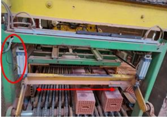
Figure 3. The location of the sensors
