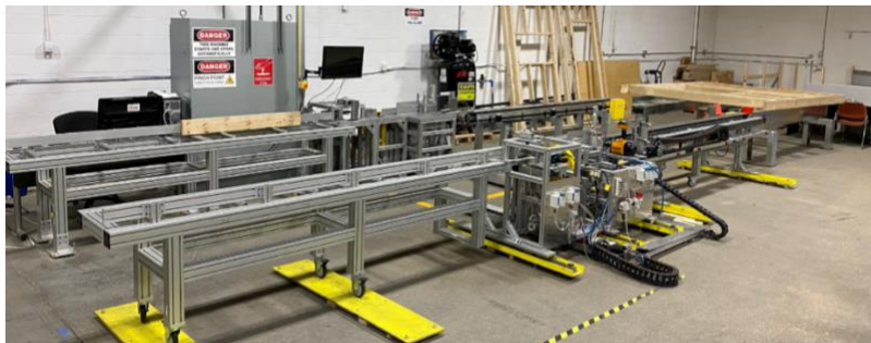
Figure 1. Wood-wall framing machine prototype at the University of Alberta lab.
